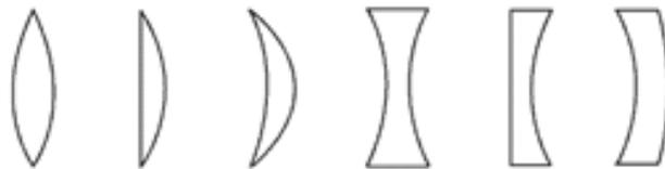
**Figure 1:** Six types of spherical lenses: biconvex, plano-convex, concave-convex, biconcave, plano-concave, convex-concave. The image is taken from [3]
