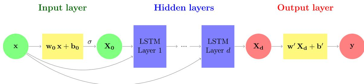
Figure 1. Architecture of DGM neural network
