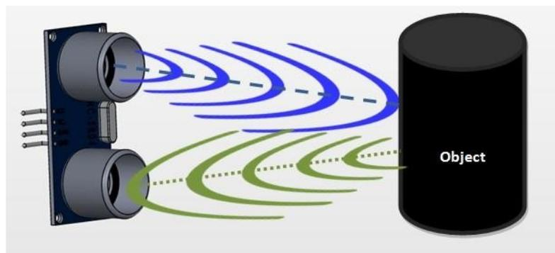
Figure 6: Ultrasonic sensor
