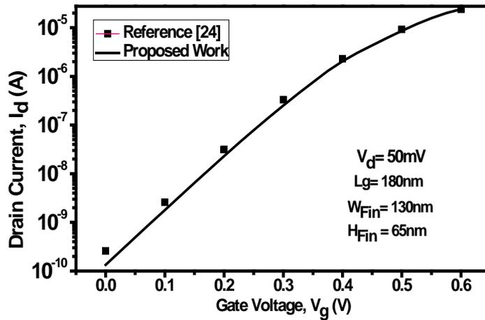
Figure 2: Transfer characteristics of proposed FINFET and reference FinFET [24]
