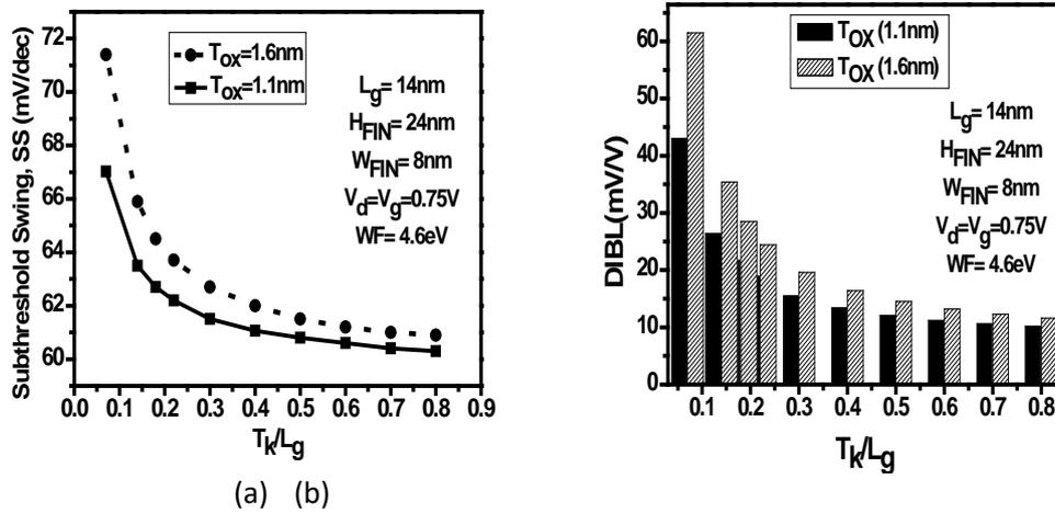
**Figure 5.** Influence of aspect ratio ( $T_k/L_g$ ) of given k dielectric permittivity on (a) SS and (b) DIBL for oxide thickness of 1.1nm and 1.6nm.
