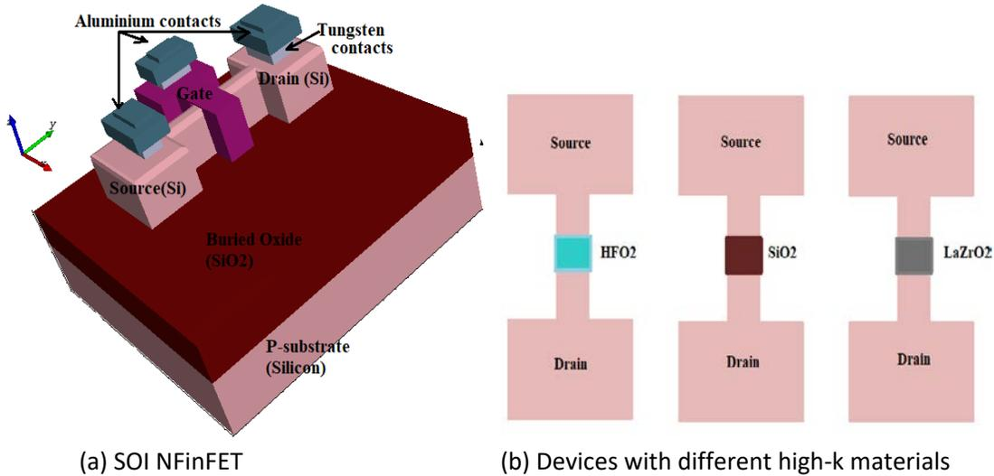
**Figure 1:** Structure of SOI NFinFET for different high-k materials
