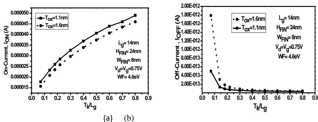
**Figure 4.** The influence of compound gate dielectric on (a)  $I_{\text{ON}}$  and (b)  $I_{\text{OFF}}$  for oxide thickness of 1.1nm and 1.6nm. (Fin aspect ratio is calculated as  $T_k/L_g = (k/3.9) \times (1.1 \text{ or } 1.6) \times (1/14)$ ).
