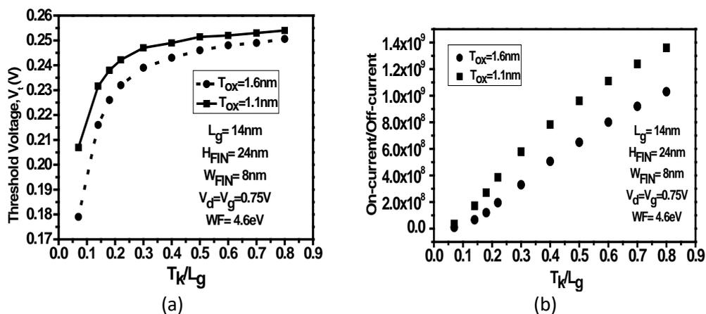
**Figure 6.** Dependence of (a)  $V_t$  and (b)  $I_{ON}/I_{OFF}$  on the aspect ratio ( $T_k/L_g$ ) for varied k of 1.1nm and 1.6nm gate oxide thickness.
