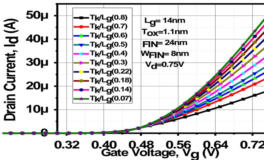
Figure 3: NFinFET Transfer characteristics for  $L_g=14\text{nm}$ ,  $k=3.9$  to  $40$ ,  $V_g=0$  to  $0.75\text{V}$  and  $V_d=0.75\text{V}$ .
