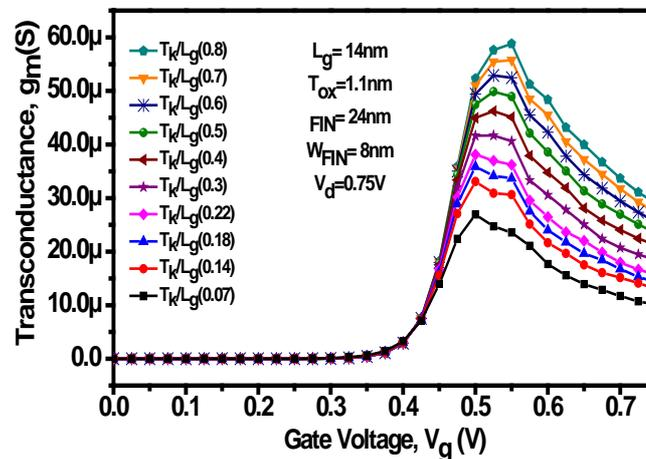
Figure 7: Transconductance trend for variable dielectric permittivity (k) of  $T_{ox}=1.1nm$ .
