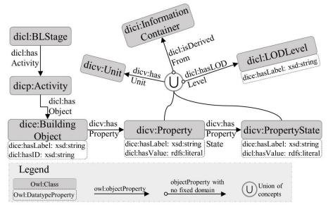
Fig. 4. LOD-sensitive BIM data representation
