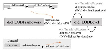
Fig. 1. Ontology-based LOD framework
