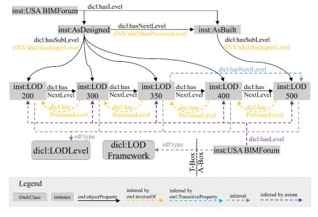
Fig. 3. Relationship between the LOD scales
