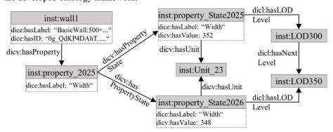
Fig. 5. Example BIM data representation at different LOD levels
