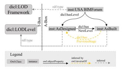
Fig. 2. Relationship between the LOD Sub-types
