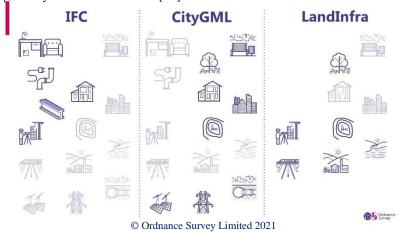
**Fig. 1.** Real-world objects represented by IFC, CityGML and LandInfra (Dark shading indicates strong coverage, light shading weaker coverage (or under development) and no shading implies no known coverage.) [32]
