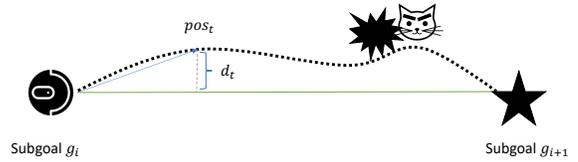
Figure 2: A demonstration on how the low-level controller executes a plan. The star is a subgoal, and the green line is the plan. The low-level controller may drift from the plan and generate the dotted path. Although our plan avoids hitting the cat, the low-level controller still cannot ensure safety during the runtime.
