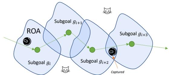
Figure 3: The way to apply the Lyapunov function. We built a sequence of ROAs around the subgoals. One ROA is a region that the robot will stay in when the robot is heading to the corresponding subgoal (i.e., the sink of the ROA). Each ROA has intersections with its neighbors.
