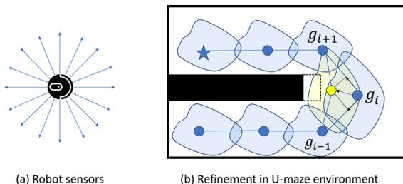
Figure 4: (a) demonstrates the sensors on the robot. The LiDARs scans 16 positions around, which generates an observation vector with 16 distance elements. (b) is an example for refinement policy. The dashed region does not exist in real world, but the map used for planning marks it as obstacle.
