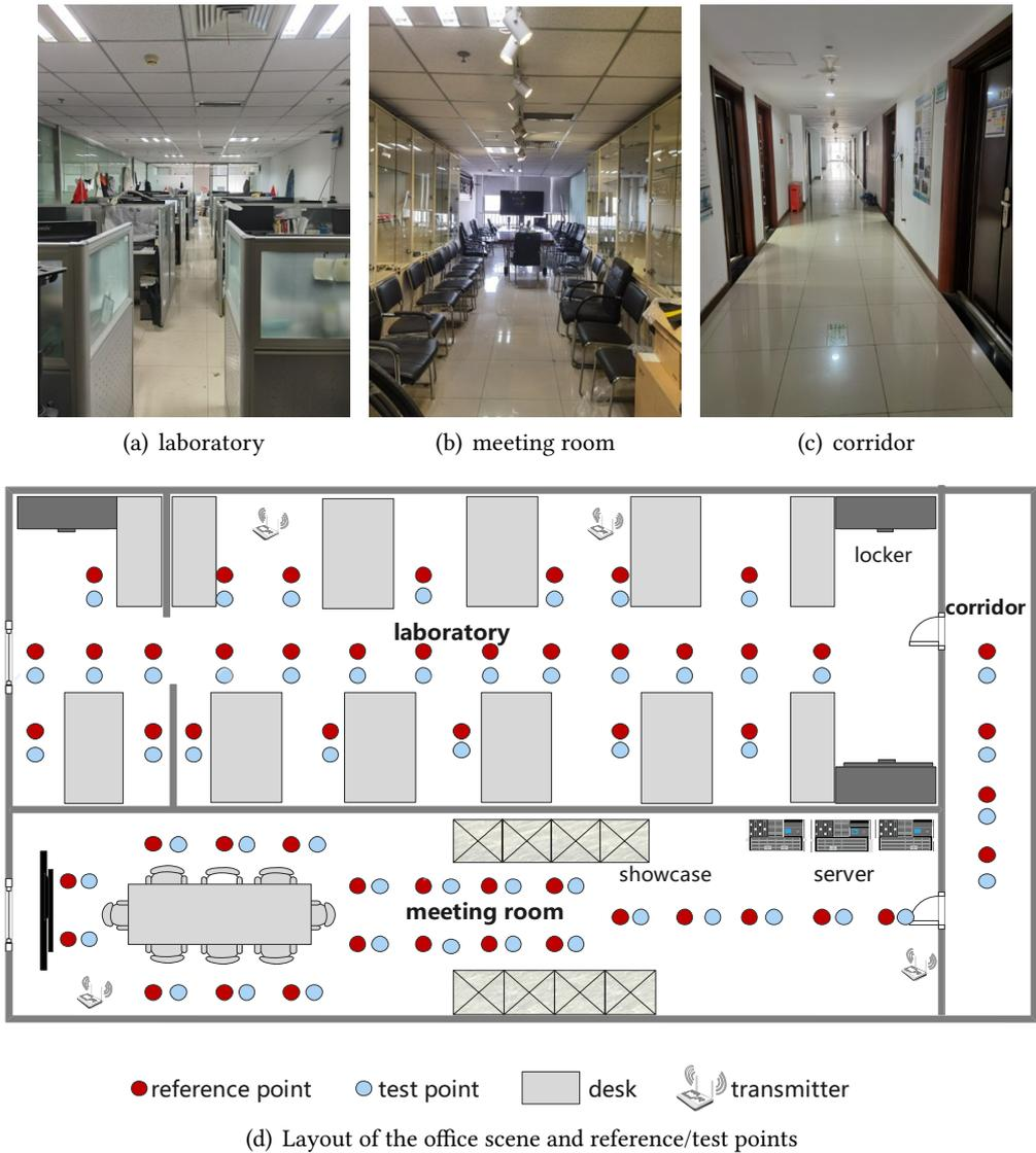
**Figure 9:** The diagram of the experiment environments.
