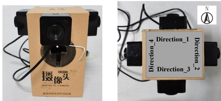
**Figure 8:** The collect equipment of multidirectional image (Left: front view, Right: top view).
