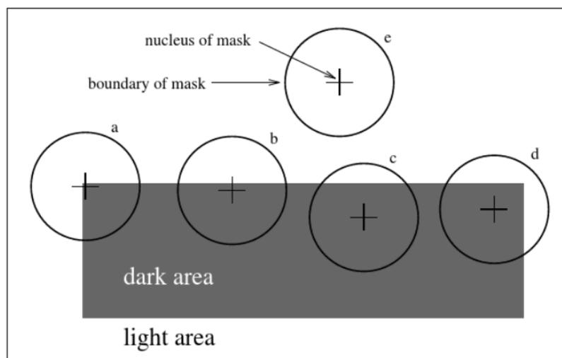
**Figure 2:** The schematic diagram of the circular window used in SUSAN[19]
