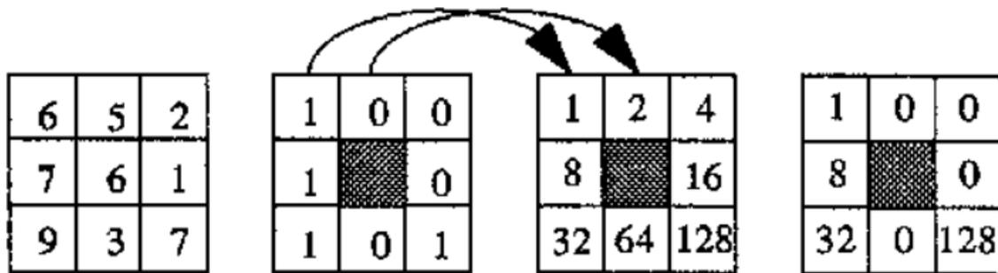
**Figure 6:** The schematic diagram of LBP algorithm when turning image intensity into binary descriptors in 3\*3 pixel neighborhood [18]
