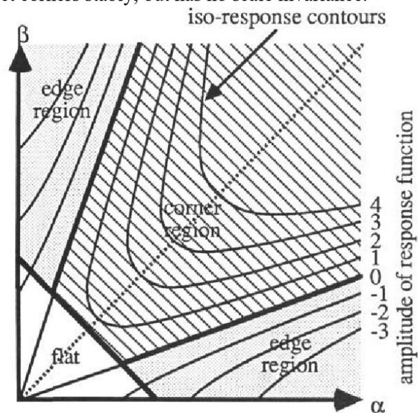
**Figure 1:** The schematic diagram of the Harris corner detection algorithm to judge the kind of zone[16]
