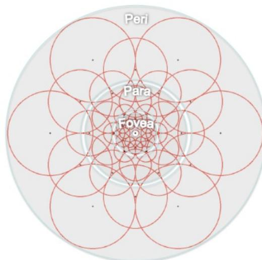
**Figure 9:** The schematic diagram of the sampling pattern used in FREAK algorithm[35]
