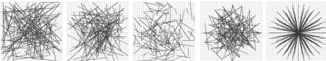
**Figure 7:** Five point-taking methods used in the BRIEF Feature Description algorithm[32]. Respectively, Uniform Distribution, Co-Parametric Gaussian Distribution, Different Parametric Gaussian Distribution, Random Sampling and Polar Point Sampling. The Co-parametric Gaussian distribution is proved to be the most effective.
