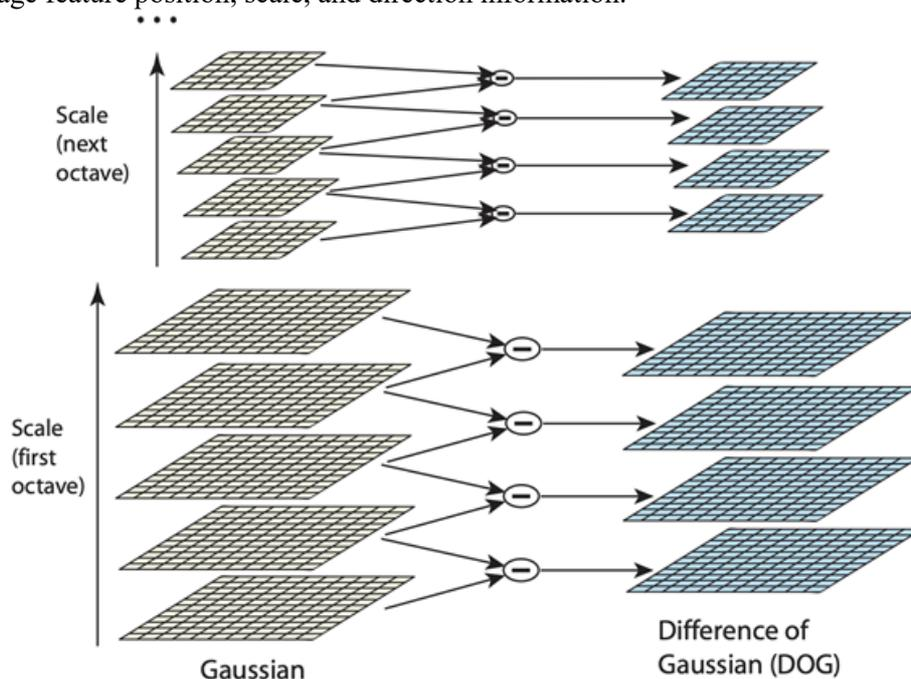
**Figure 4:** Gaussian scale space used in SIFT[23]
