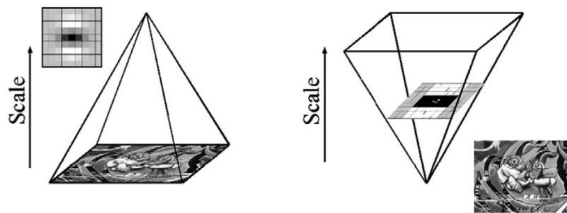
**Figure 5:** Instead of iteratively reducing the image size (left), the use of integral images allows the up-scaling of the filter at constant cost (right).used in SURF[26]
