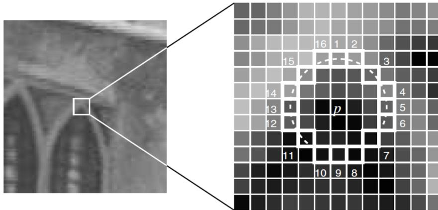
**Figure 3:** The Schematic diagram of sampling area when FAST feature detection algorithm extracts features[21]
