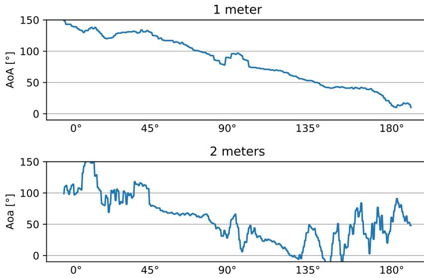
**Figure 9:** Outdoor AoA measurements at different distances with respect to the real angle.
