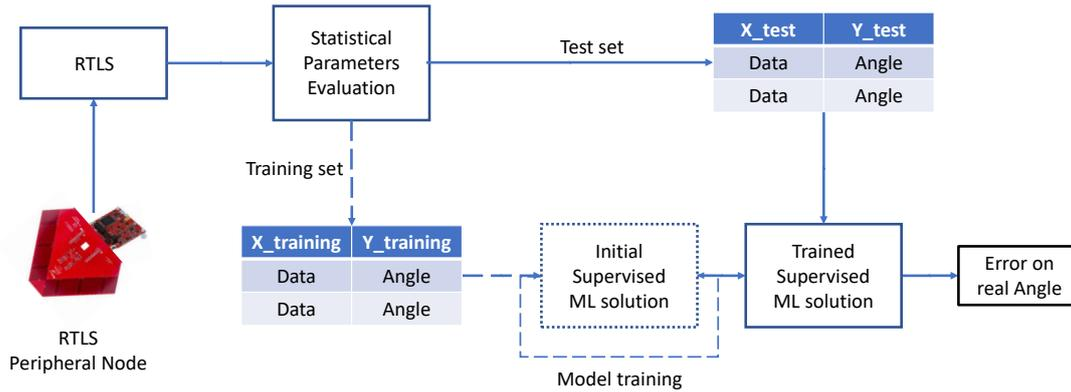
**Figure 4:** High-Level representation of the proposed Framework for AoA evaluation and error calculation.
