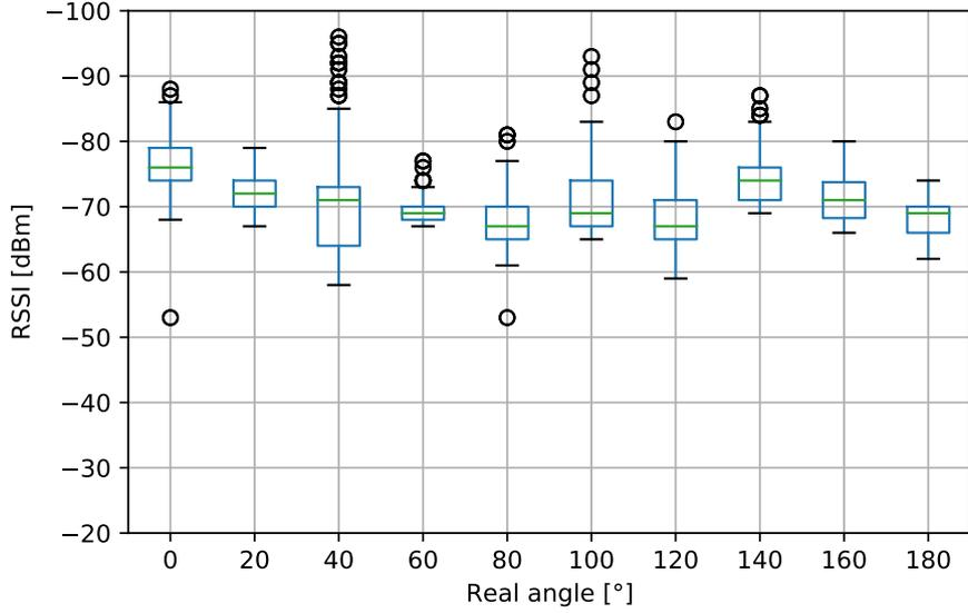
**Figure 8:** Indoor RSSI measurements at 3 m distance.
