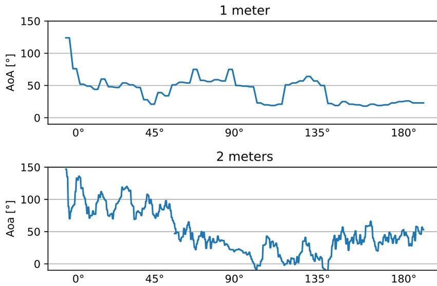
**Figure 10:** Indoor AoA measurements at different distances with respect to the real angle.
