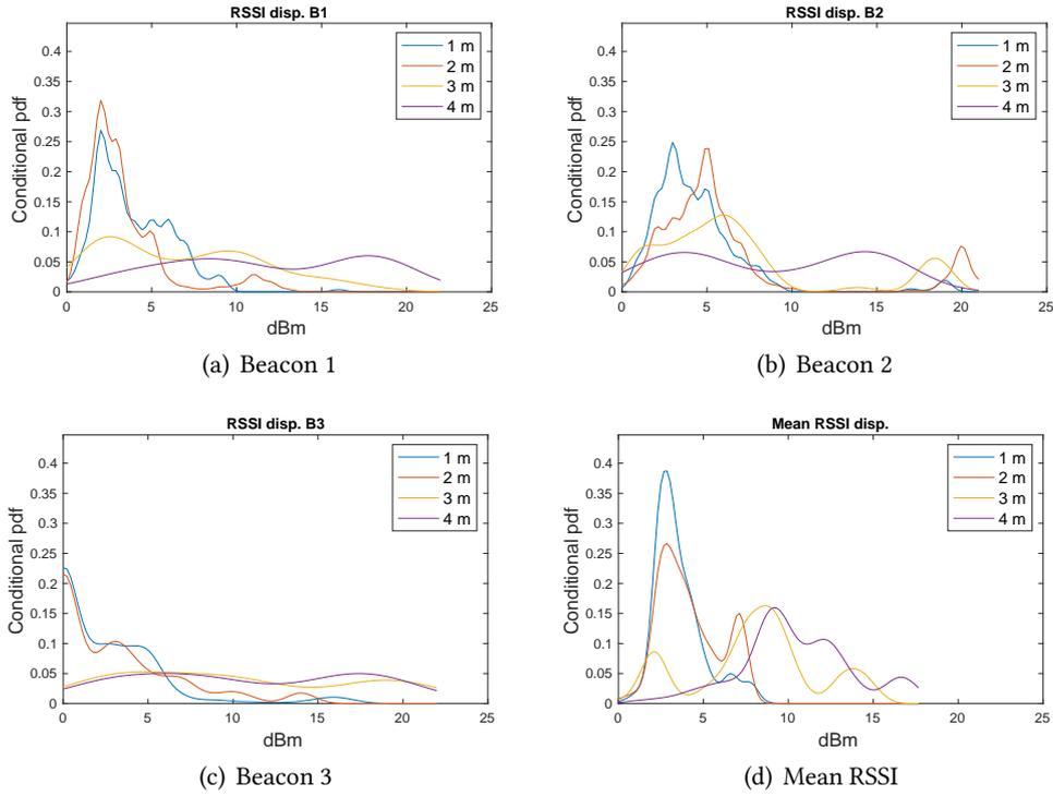
**Figure 4:** The pdf of the measured RSSI disparity, conditioned on the four different interpersonal distances considered (Home data collection). The last plot refers to the mean of the RSSI disparity over the three beacons.
