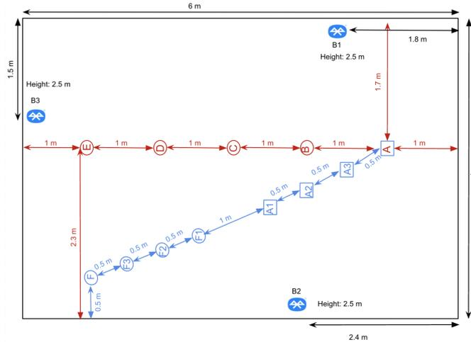
**Figure 2:** Home data collection layout: Set 1 data collection at (A1, F1), (A2, F2), (A3, F3), (A, F) location pairs at 1, 2, 3, and 4 meters interpersonal distance respectively. Set 2 and Set 3 data collection at (A, B), (A, C), (A, D), (A, E) location pairs at 1, 2, 3, and 4 meters interpersonal distance respectively. For Set 2 and 3, one experimenter stood still in position A, while the second experimenter moved in turn on the other locations.
