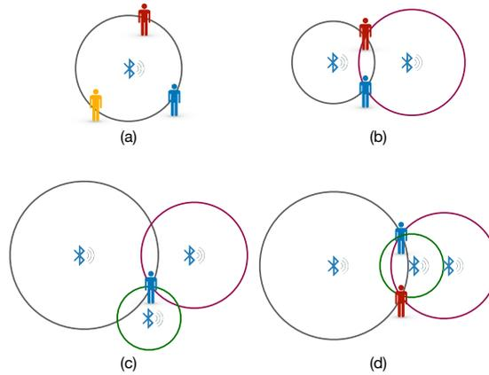
**Figure 1:** Examples of ambiguous zero RSSI disparity situations using one beacon (a), two beacons (b), and three or more collinear beacons (d). Ambiguity can be avoided by using three or more non-collinear beacons (c). These examples assume isotropic signal loss and uniform emission power.
