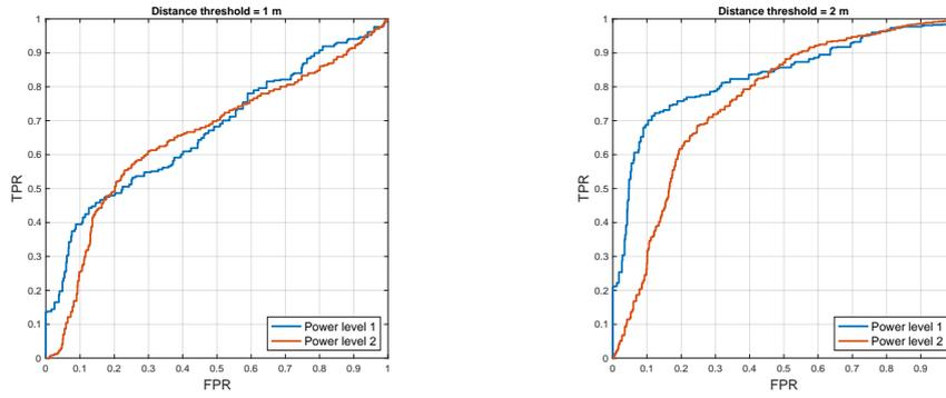
**Figure 10:** ROC curves using mean RSSI disparity for proximity detection at distance thresholds of 1 m and 2 m. Shuttle data collection at BLE power level 1 (blue curve) and at BLE power level 2 (red curve).
