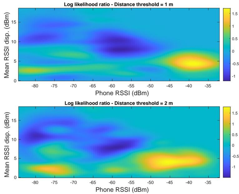
**Figure 8:** The log likelihood ratio of the vector formed by phone RSSI and mean RSSI disparity, conditioned on the interpersonal distances being smaller (null hypothesis) or larger (alternative hypothesis) than the considered threshold of 1 m or 2 m (Shuttle data collection at BLE power level 1 and 2).
