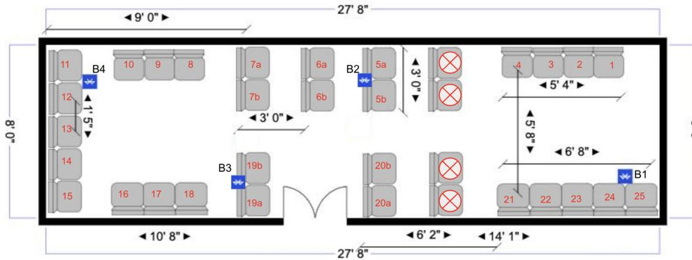
**Figure 7:** Shuttle data collection layout representing the location of the beacons deployed on the shuttle ceiling and seat numbers. Right of the figure is the front of the shuttle. Crossed red circle seats are blocked seats for COVID-19 distancing.
