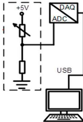
**Figure 4.** Voltage divider circuit [9]
