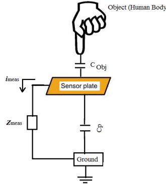
**Figure 5.** The circuit of capacitive sensor [11].
