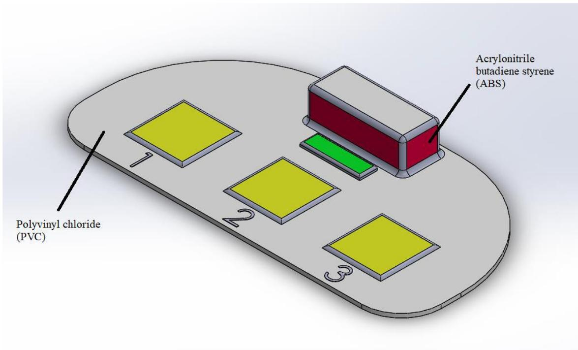
**Figure 2.** Design of the tactile mat.
