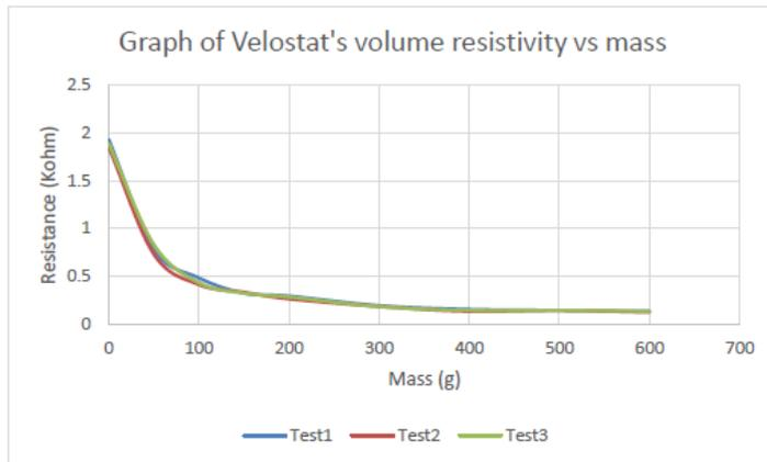
Figure 4. Graph of Velostat's volume resistivity vs mass.
