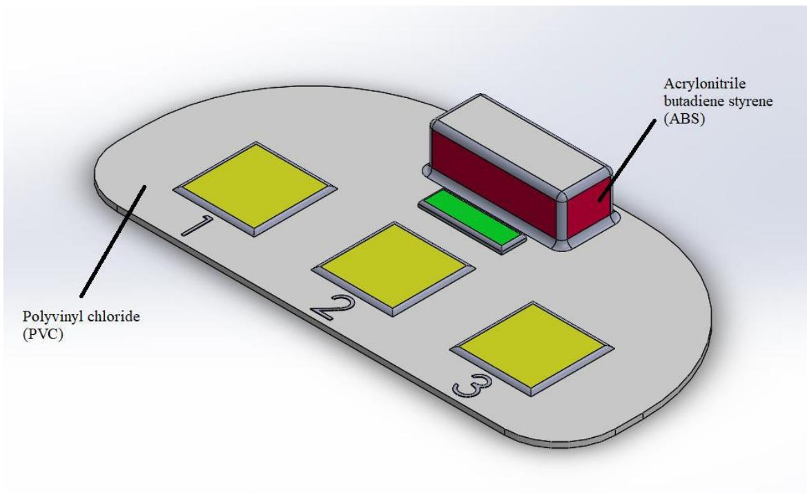
**Figure 2.** Design of the tactile mat.
