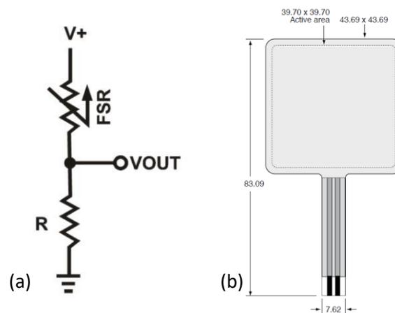
**Figure 3.** (a) Voltage divider with FSR sensor, (b) FSR01.
