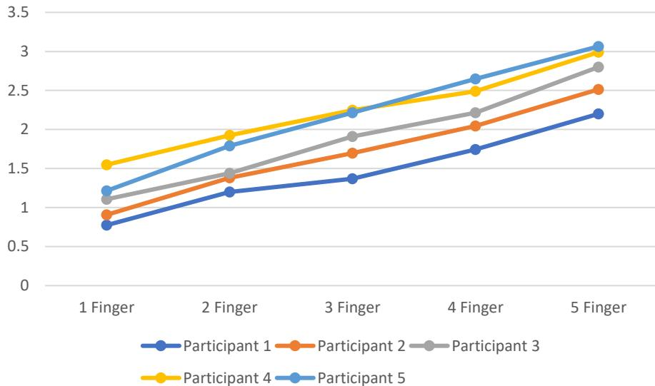
**Figure 9.** Graph of Average voltage reading (V) vs. Number of Fingers.
