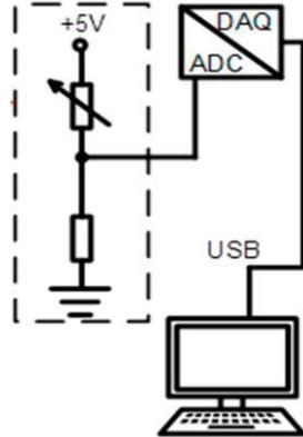
**Figure 4.** Voltage divider circuit [9]
