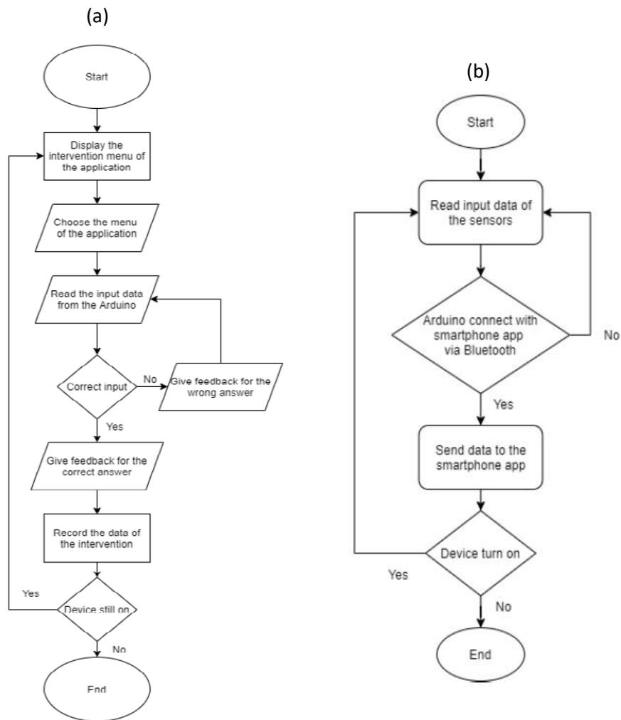
**Figure 3.** (a) Flowchart of the hardware, (b) Flowchart of the mobile application.
