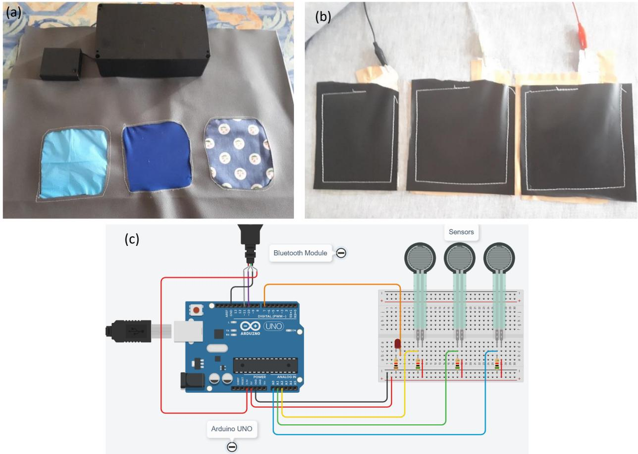
**Figure 5.** (a) Prototype of the device, (b) The Velostat of the tactile mat, (c) Circuit configuration
