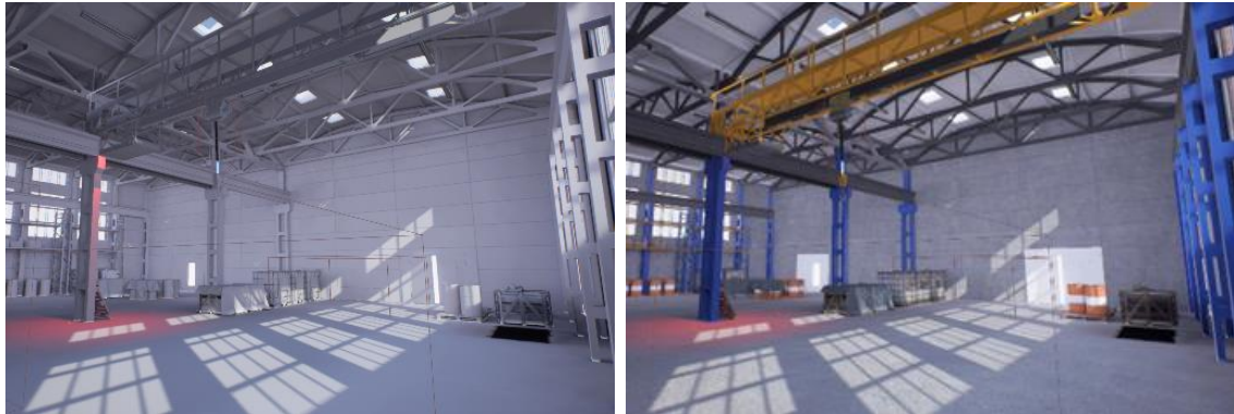
Figure 1: The Virtual Reality Overhead Crane Simulator. The 3D model without materials (left). The 3D model with physically based rendering materials (right).
