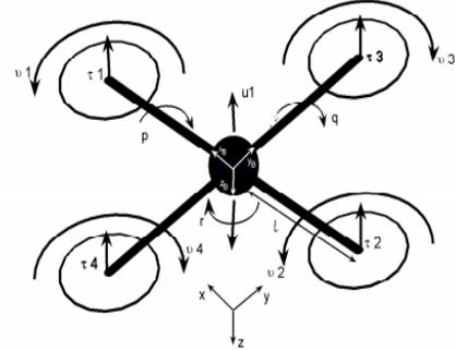
Figure 1. Quadrotor Schematic
