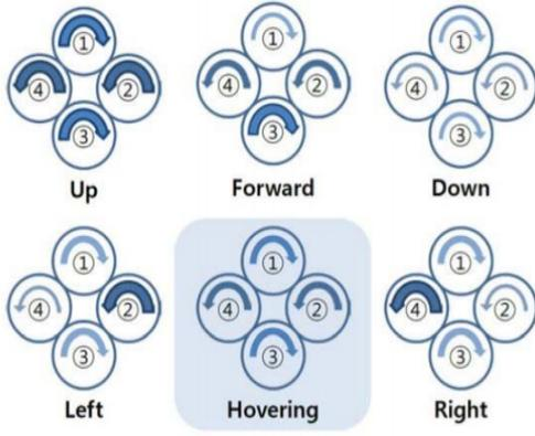
Figure 2. Mechanism of Quadrotor movements
