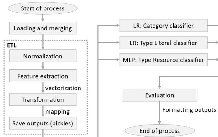
**Fig. 8.** System workflow chart of the final CitySAT. One of the key algorithms is for data transformation and mapping the intended number of types in the experiments looping sub-process in type classification (partially retrieved code is stated in Appendix).
