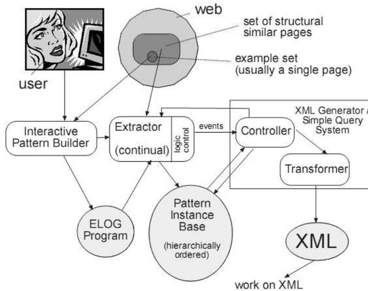
Fig. 1. The architecture of *LiXto*, from [7]
