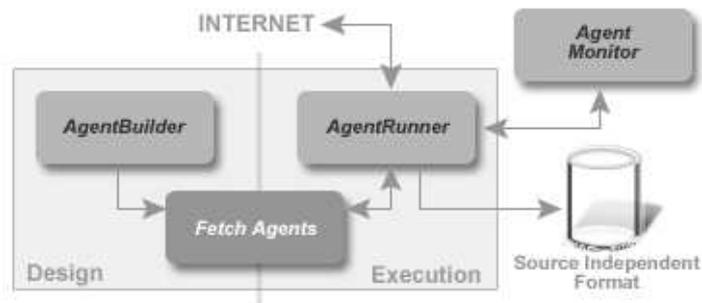
Fig. 2. The architecture of *Fetch Agent Platform*, from [21]
