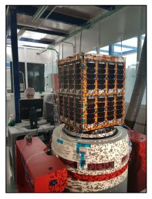
Figure 1. The UPMSat-2 satellite during vibration tests at the IDR/UPM Institute facilities at the Montegancedo Campus (Madrid).
