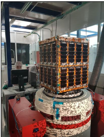
Figure 1. The UPMSat-2 satellite during vibration tests at the IDR/UPM Institute facilities at the Montegancedo Campus (Madrid).
