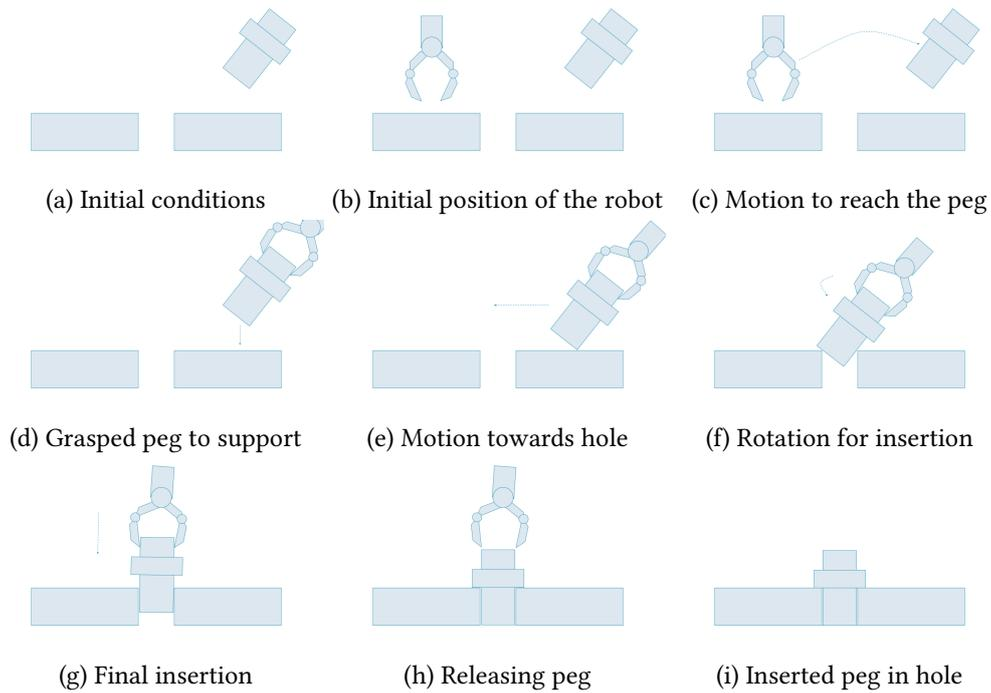
**Figure 3:** Various stages of a peg-in-a-hole skill. The robot needs to grasp a peg and successfully insert it into the respective hole. Initially the robot grasps the peg and moves it towards the surface that has the hole until there is contact 3a-3d. Then it moves the peg towards the hole until the motion is blocked by the peg being partly inserted 3e. Finally, the peg is rotated, inserted, and released 3f-3i.
