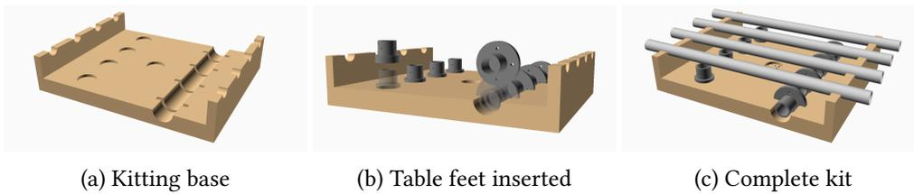
**Figure 2:** Various stages of a kitting application. The base is supporting the other elements of the table. Feet and legs are inserted having precedence and position constraints.
