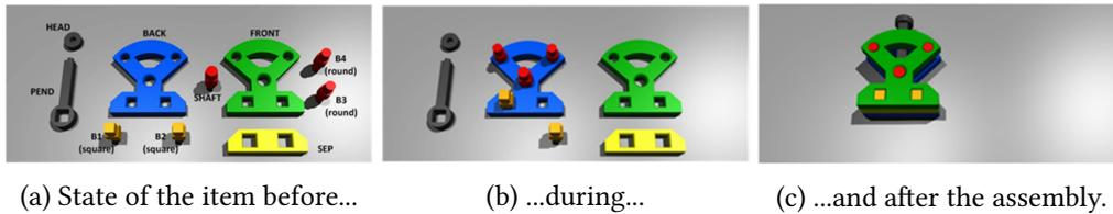
**Figure 1:** The Cranfield assembly task in various stages of execution. This task is used as a benchmark for testing solutions to the automated assembly problem using robots [13].
