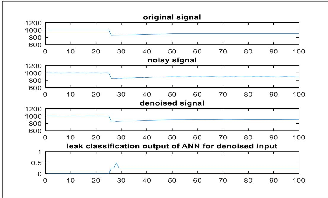
**Figure 3:** original, noisy, and denoised signals with classification result for the ANN output
