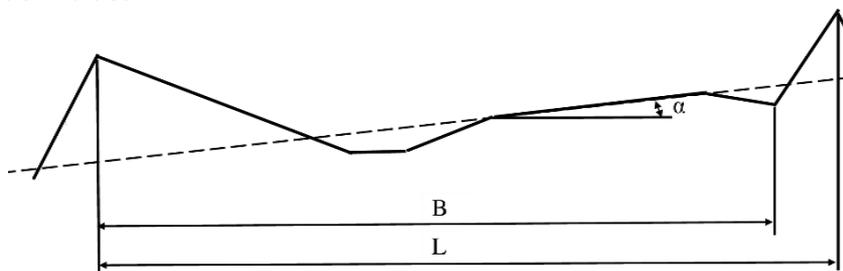
**Figure 2:** The cross-section of rampart-terrace surface  $\Gamma$  (B — the width of the strip of agricultural use, L — the distance between the ramparts,  $\alpha$  — the angle of inclination of the surface of the segment)
