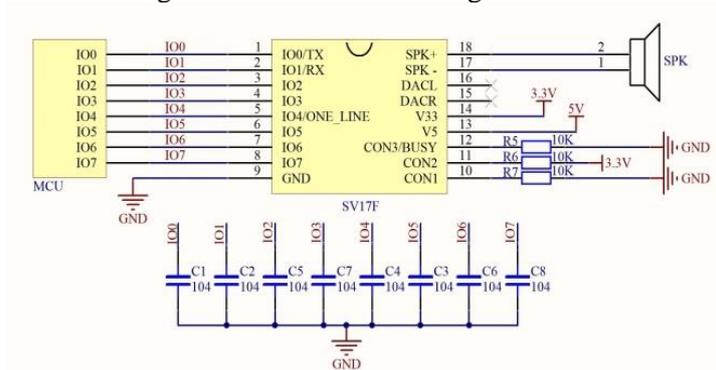
**Figure 4:** Voice module connection diagram
