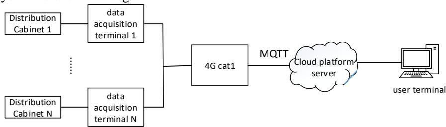
**Figure 1:** Overall architecture diagram of monitoring system
