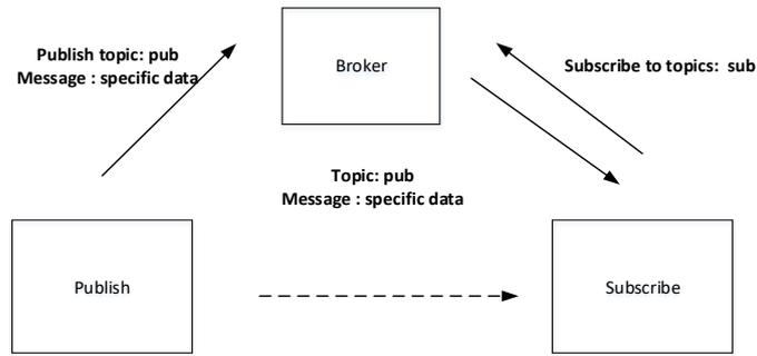
**Figure 7:** MQTT work flow chart
