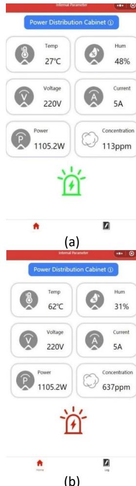
**Figure 8:** (a) Data normal interface, (b) Data exception interface, (c) SMS interface.
