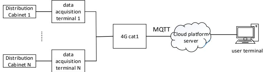
**Figure 1:** Overall architecture diagram of monitoring system
