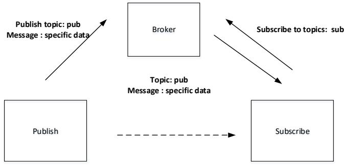
**Figure 7:** MQTT work flow chart
