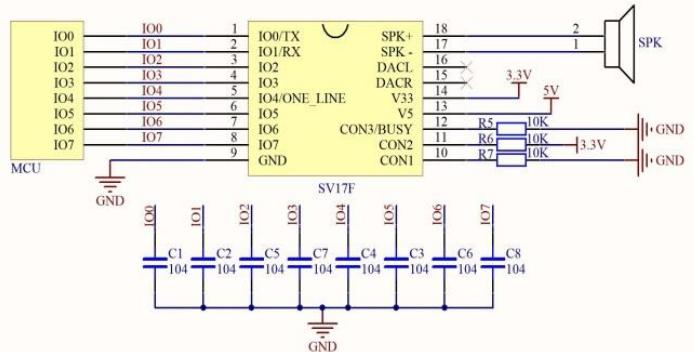
**Figure 4:** Voice module connection diagram
