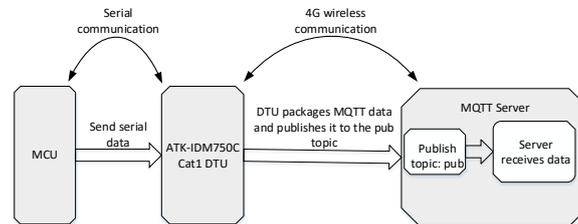
Figure 5: Schematic diagram of data transmission
