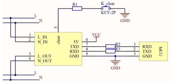
**Figure 2:** Connection diagram of SUI-101A and MCU
