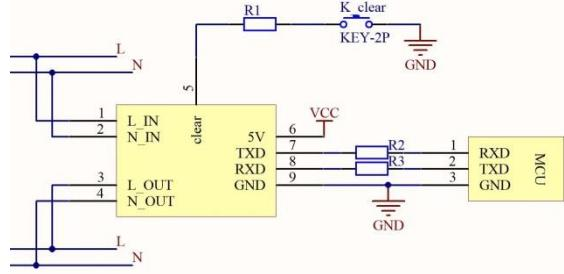
**Figure 2:** Connection diagram of SUI-101A and MCU
