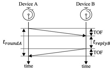
Figure 3: TWR mechanism [31].
