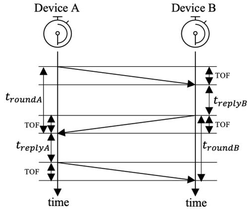
Figure 4: Symmetric TWR mechanism [31].
