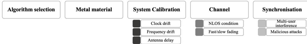
**Figure 5:** Overview of all potential ranging/positioning error in terms of the TOF, TDOA and AOA technique performed by UWB.
