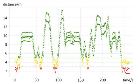
**Figure 10:** Distance between the Target 2 and one of the vehicle anchor (2nd experiment).
