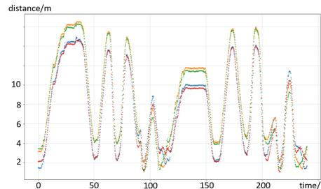
**Figure 8:** Distance between the target and one of the vehicle anchors (1st experiment).
