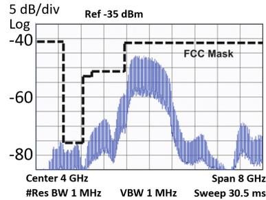
**Figure 1:** Typical transmitted power spectral density of UWB signal.
