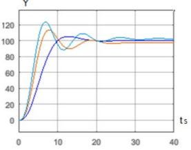
**Figure 4**: Transient characteristics of the system while increasing the transmission coefficient of the object at the initial system when  $k_0$ =10 the overshooting is 5%
