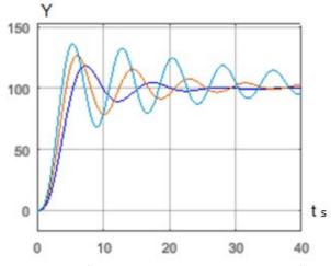
**Figure 5**: Transient characteristics of the system with the increase of the transmission coefficient of the object
