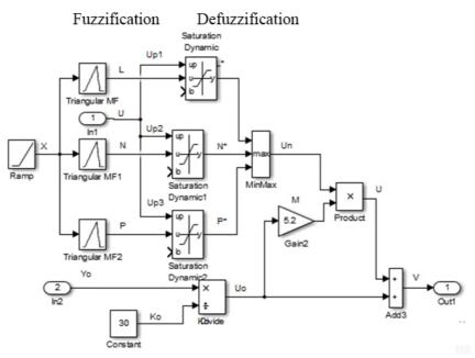
Figure 2: The scheme of the fuzyfication and defuzyfication units
