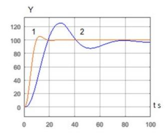
**Figure 6:** Transition characteristics of the system when decreasing and increasing of the time constant of the object
