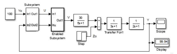
Figure 1: Scheme of fuzzy control system with fuzzy PD-controller
