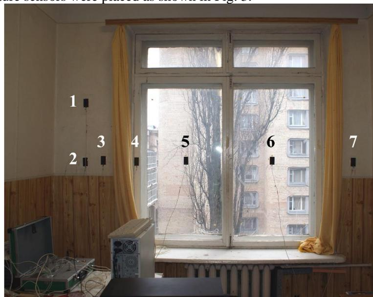
**Figure 3:** The heat flux and temperature sensor's location in the test room
