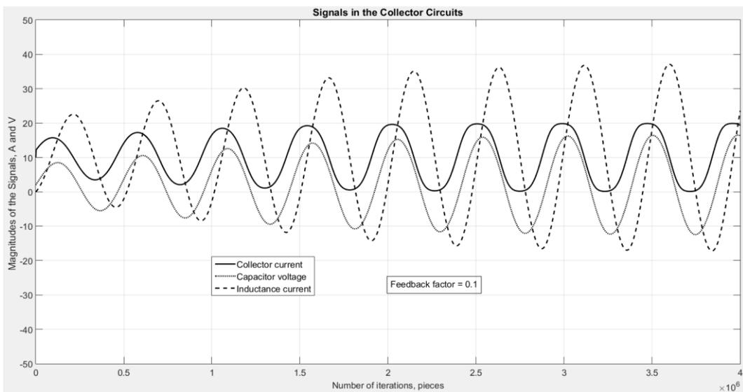
**Figure 13:** Collector current, capacitor voltage and inductance current for the feedback factor 0.1
