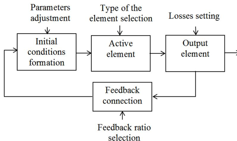
**Figure 1:** Information flow and the controlling inputs in the oscillator
