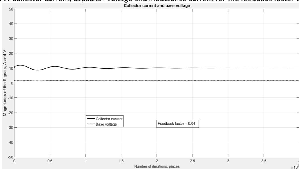
**Figure 8:** Collector current and base voltage for the feedback factor 0.04
