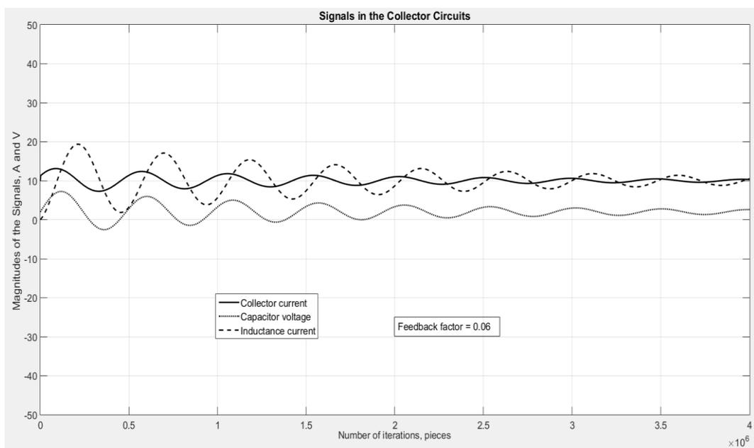
Figure 9: Collector current, capacitor voltage and inductance current for the feedback factor 0.06
