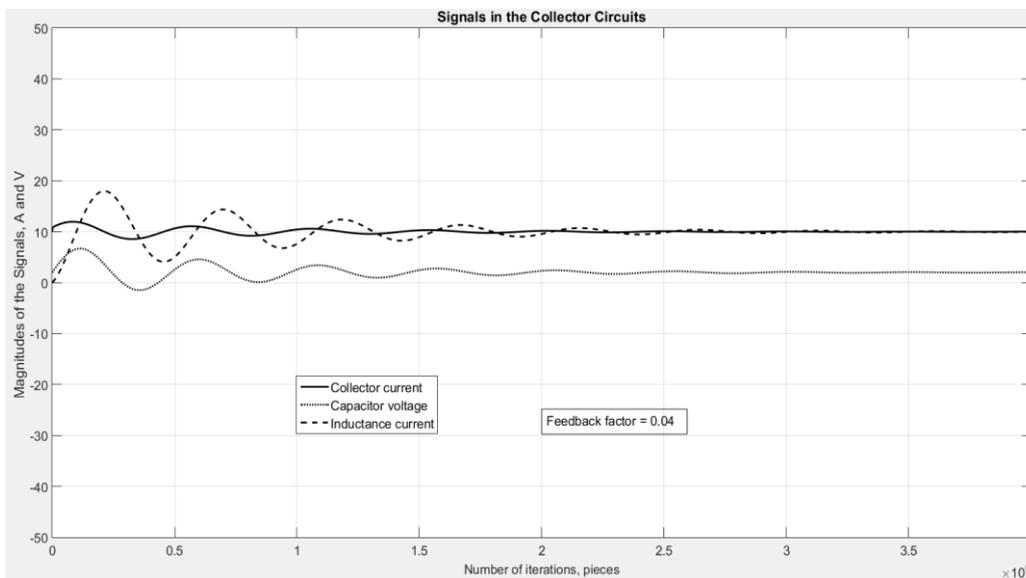
**Figure 7:** Collector current, capacitor voltage and inductance current for the feedback factor 0.04
