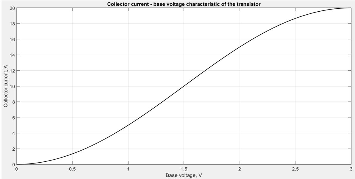
**Figure 2:** Collector current-base voltage characteristic of the transistor
