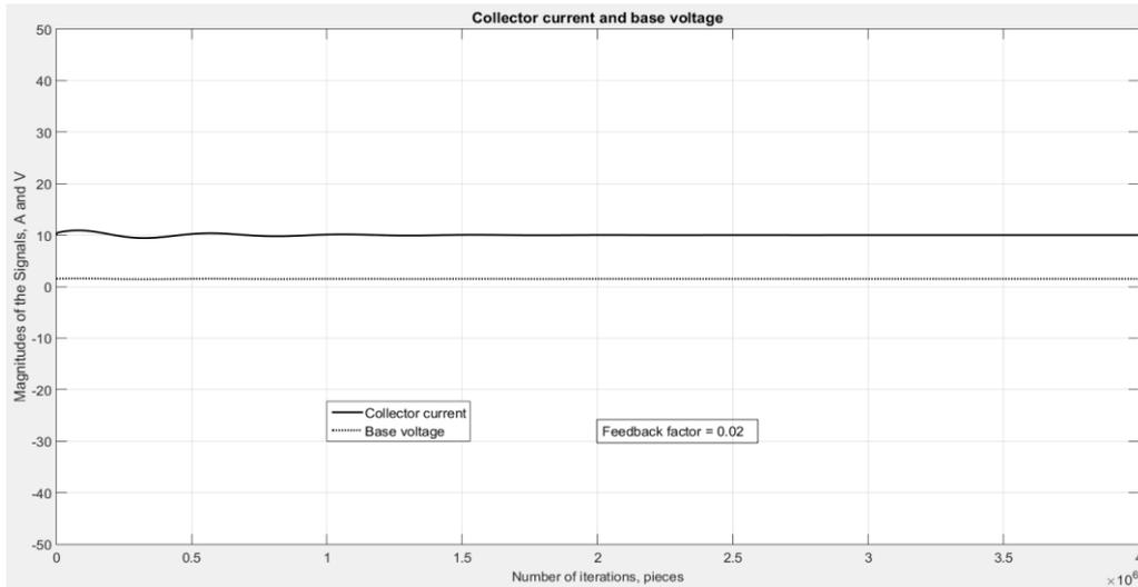
**Figure 6:** Collector current and base voltage for the feedback factor 0.02
