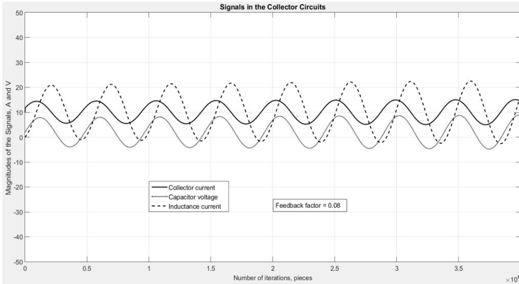
**Figure 11:** Collector current, capacitor voltage and inductance current for the feedback factor 0.08
