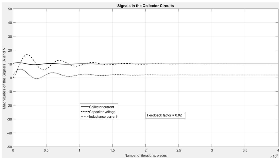
**Figure 5:** Collector current, capacitor voltage and inductance current for the feedback factor 0.02
