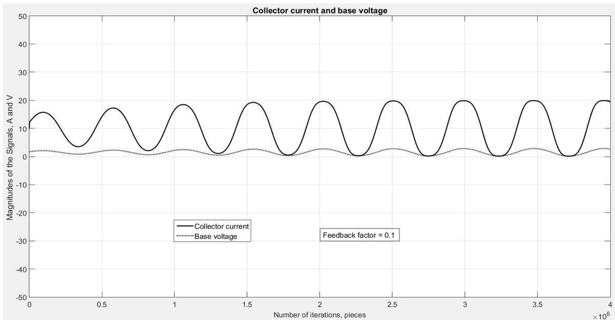
**Figure 14:** Collector current and base voltage for the feedback factor 0.1
