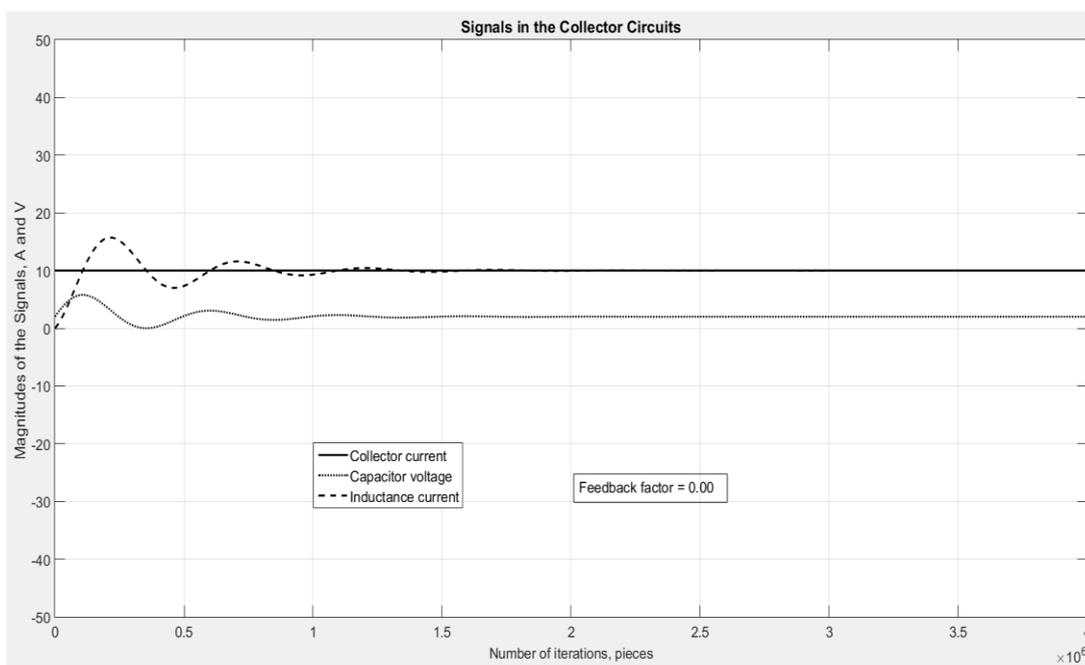
**Figure 3:** Collector current, capacitor voltage and inductance current for the feedback factor 0
