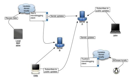
Fig. 2. Global architecture of distributed semantic microblogging
