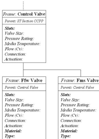
**Fig. 5.** A partial view of the component hierarchy. It shows the frame for a *control valve* and two subtypes: *Ffw* and *Fms* valves.
