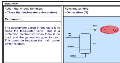
Fig. 2. An example of an explanation defined by a domain expert.
