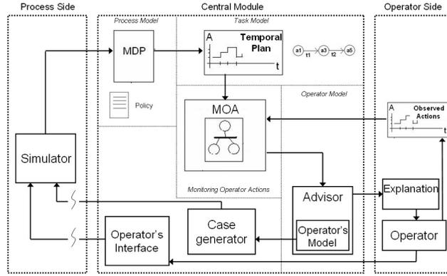
**Fig. 1.** IAOT block diagram [2]. It consists of 3 main parts: process side (simulator), operator side and the central module. Based on the optimal policy obtained from the MDP a temporal plan is generated. The operator actions are compared to the plan (MOA) and according to this the Advisor generates explanations.
