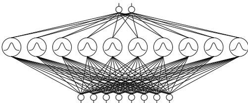
**Fig. 2.** A scheme of a Radial Basis Function Network.
