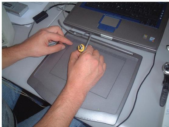
Figure 2. Experimentation of the AudioTact™ device: a visually impaired user explores the virtual image using the left hand for spatial references and the right hand for scanning for aural and vibrational cues.
