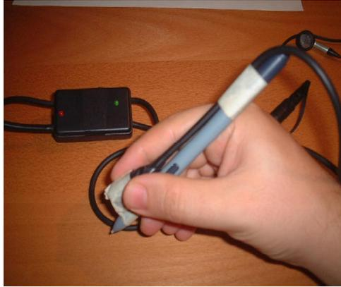
Figure 1. Experimentation of the AudioTact™ device: a picture of a pen with the vibro-audio device attached.
