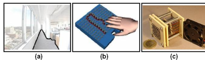
Figure 3, (a) information about the environment obtained from cameras and image processing, (b) tactile representation of the environment, (c) the tactile device (TactiPad, ISIR, University of Paris 6).
