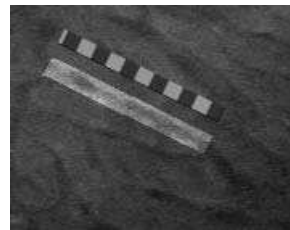
Fig. 3. Sinusoid section, dynamic pattern to estimate velocity ground truth.
