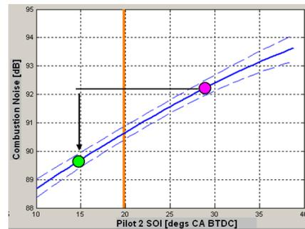
Fig. 11 Pilot timing effect on the noise model
