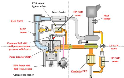
Fig. 1 Test-engine with replaced Engine Management System (EMS)
