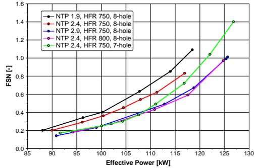
Fig. 6 Selection of NTP, HFR and no. of holes
