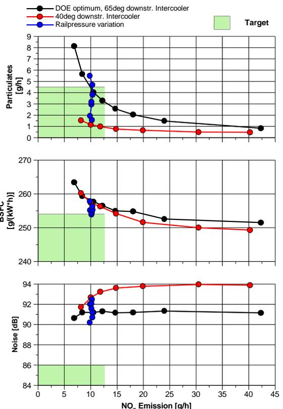
Fig. 7 Effects of intake charge cooling and rail pressure variation on performance
