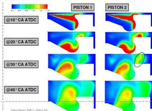
Fig. 9 Comparison of equivalence ratio distribution between piston 1 and 2 design
