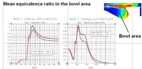
Fig. 10 Post-processed distribution of fuel vapor between bowl and squish area
