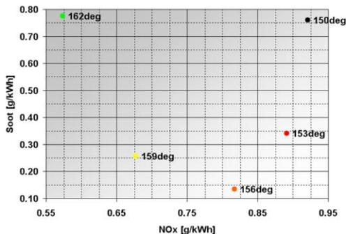
Fig. 5 Variation of spray cone angle
