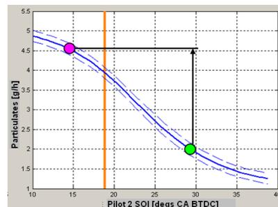
Fig. 12 Pilot timing effect on the soot model
