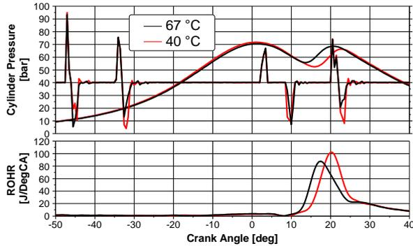
Fig. 8 Effect of intake charge cooling
