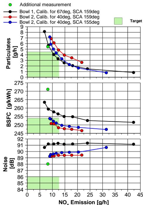
Fig. 13 Engine performance of piston 2 bowl design
