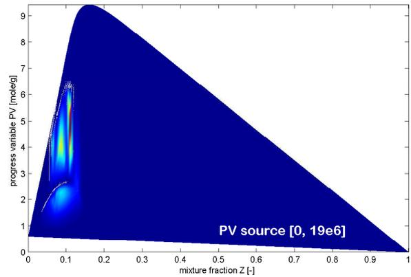
Figure 2: Igniting flamelet manifold.  $PV$  source as function of  $Z$  and  $PV$ .
