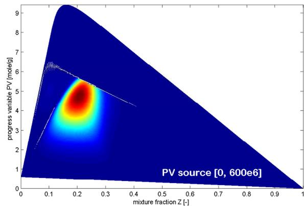
Figure 3: Homogeneous reactors manifold.  $PV$  source as function of  $Z$  and  $PV$ .
