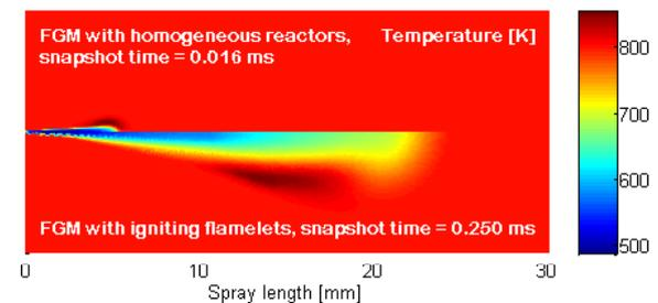
Figure 4: Temperature contours. At start of injection the time is 0 ms and the ambient temperature is 800 K.
