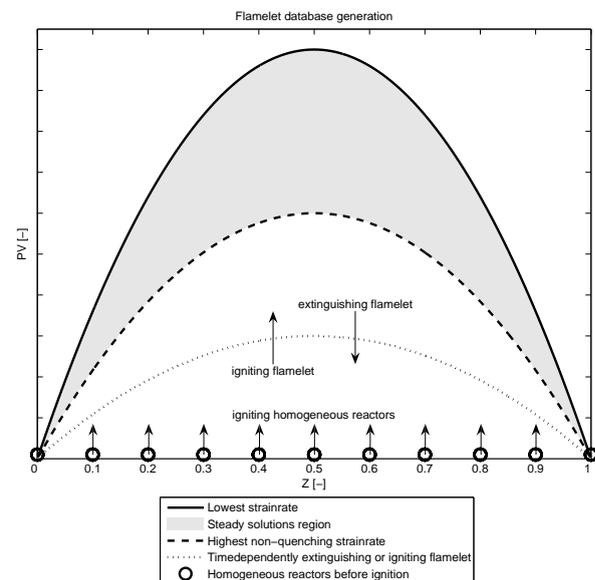
Figure 1: Ways to extend a stationary database
