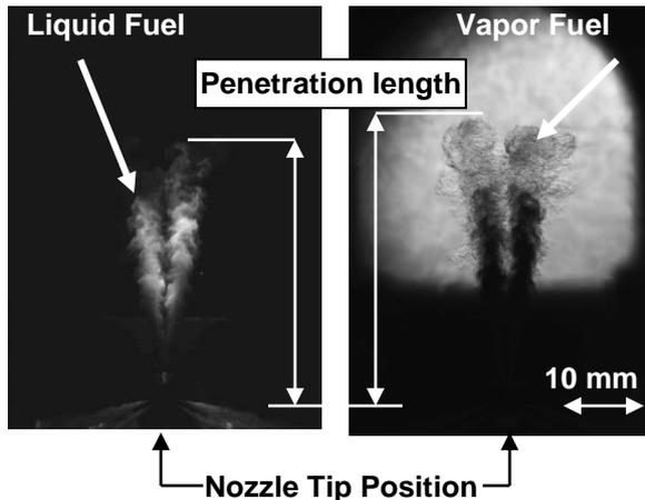
Fig. 1: Sample images of the sprays from a 15° cluster nozzle,  $p_{rail} = 600$  bar,  $t_{aei} = 1000$   $\mu$ s. Determination of penetration length, (Left) Mie-Scattering for liquid phase and (Right) Schlieren for vapor phase.
