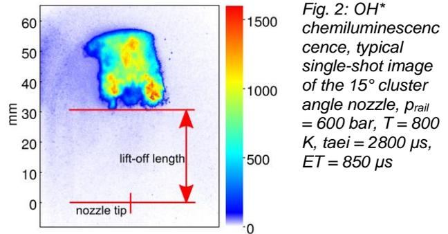
Fig. 2: OH\* chemiluminescence, typical single-shot image of the 15° cluster angle nozzle,  $p_{rail} = 600$  bar,  $T = 800$  K,  $t_{aei} = 2800$   $\mu$ s,  $ET = 850$   $\mu$ s
