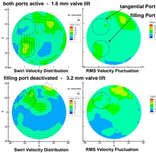
Figure 3: Charge motion analysis by 3D PIV without and with filling port deactivation at  $z = 75$  mm
