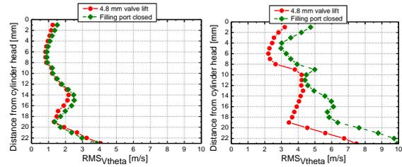
Figure 7: RMS value of tangential velocity using RANS(left graph) and LES(right graph)
