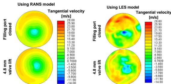
Figure 6: Cut section of the tangential velocity field in the middle of the bowl using the RANS model (left) and the LES model (right) at -30°CA ATDC
