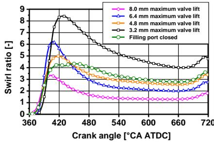
Figure 5: Swirl ratio over crank angle as calculated by RANS CFD simulations.
