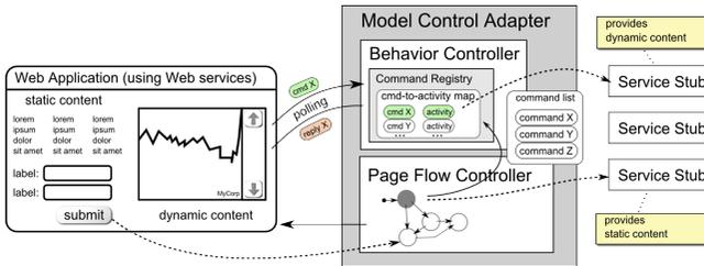
**Fig. 2.** UI- to Service-interaction within the reference architecture
