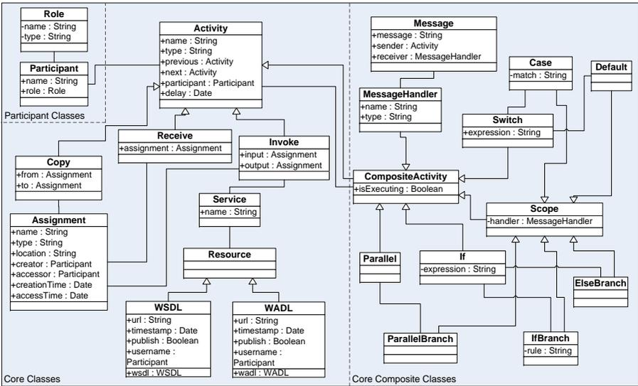
Fig. 3. The Service Mashup Abstraction represented using UML
