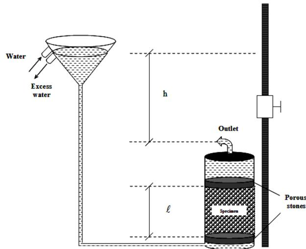
Fig. 1. The combination permeameter- constant head situation.
