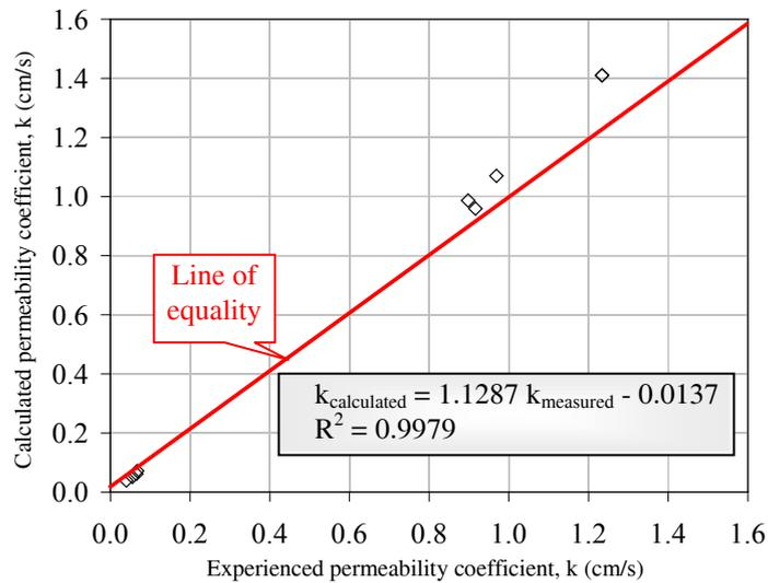
Figure 7. The comparison of calculated and experienced permeability coefficients.
