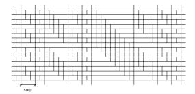
Figure 1: Bitonic sorting networks for 16 elements. Each step is completed when all comparisons involved are computed. In the figure each comparison is represented with a vertical line that link two elements, which are represented with horizontal lines.
