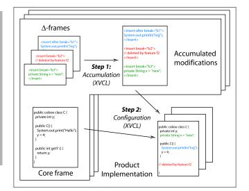
Figure 7. Automated Product Derivation using XVCL
