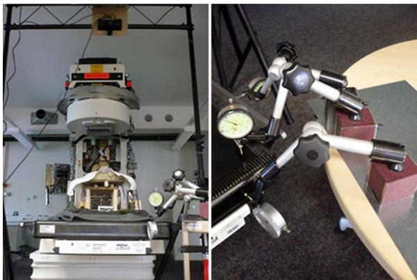
**Fig. 3.** Test setup: left side: Siemens ONCOR system with ToF camera viewing the body plaster cast phantom; right side: three measurement gauges to measure patient table displacement with an accuracy of 1/100 mm.
