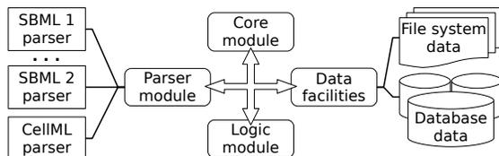
**Fig. 1.** System components are integrated to work together preserving a flexible and easily extensible architecture. Each module has different versions used on the basis of job in progress (*e.g.*, to parse an SBML file, will be dynamically chosen the SBML parser).
