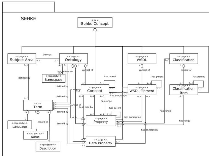
Figure 2: Schema of system concepts of SEHKE environment
