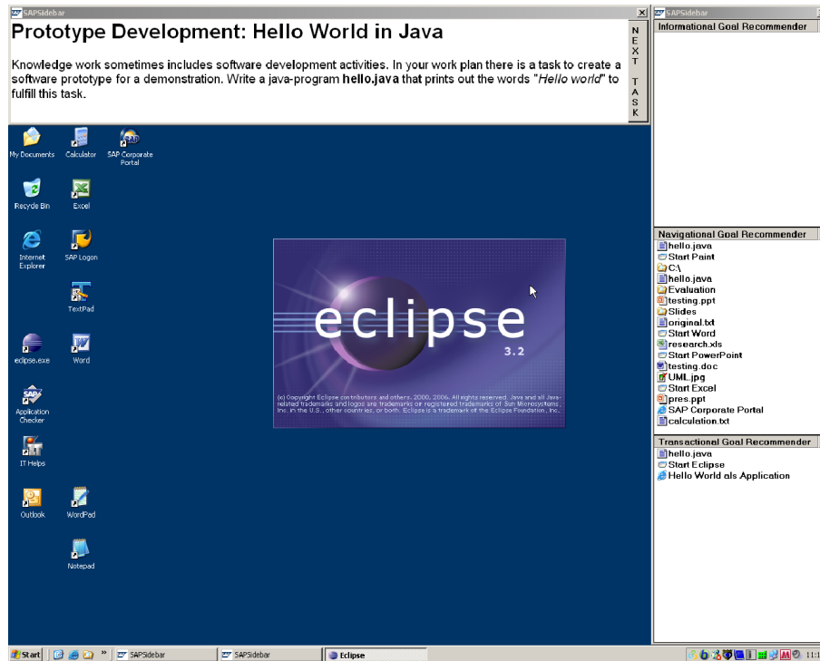
Fig. 3. Screenshot of the simplified UI - the right hand sidebar showing three potential recommended list of documents from topic detection (with a topic as informational goal), purely unsupervised mechanisms based on the users clickstream (a document or URL as a navigational goal) and task detection (with a task as transactional goal).
