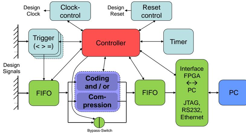
**Fig. 2.** Architecture of the on-chip debugger modules
