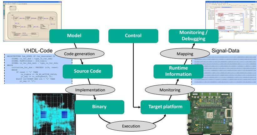
Fig. 1. Design flow for model-based monitoring and control [10],[14],[16]
