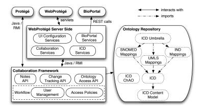
**Fig. 1.** An architecture diagram of WebProtégé used in the ICD context. WebProtégé front-end uses the services in the WebProtégé server side to display information to the user. The WebProtégé server side and the desktop client Protégé connect to the *Collaboration Framework* to access the ontology and the collaboration services. The *Ontology Repository* stores the ontologies available to the clients.
