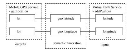
Fig. 1. Since the output parameters ("lat" and "lon") of operation "getLocation" have the same semantic annotations ("geo.latitude" and "geo.longitude") as input parameters ("latitude" and "longitude") of operation "addPushpin", Mobile GPS service is linkable to Virtual Earth service.
