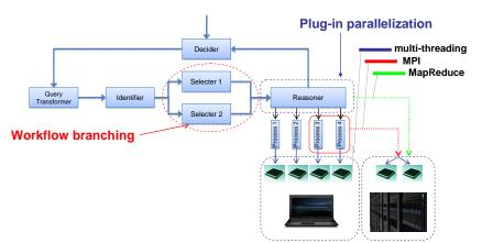
**Fig. 1.** For the semantic applications, which are described through complex workflows, parallelization can be applied on different levels: workflows (task- and data-level parallelism), or single components/plug-ins (data- and instruction-level parallelism).
