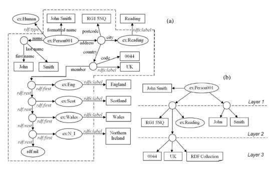
Fig. 2. The unit-graph for a resource that contains blank nodes and RDF collection
