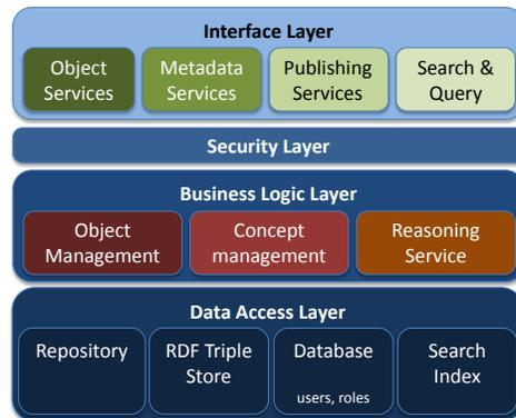
**Fig. 1.** A high-level depiction of components in the ontology-driven architecture.
