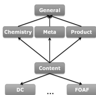
The general ontological model of ChemCloud is composed of a set of modular ontologies: General ontologies cover more common concepts from the application domain such as content, product and term, while specialized domain ontologies describe concepts such as thermophysical and thermochemical properties, reactions and compound classes.
