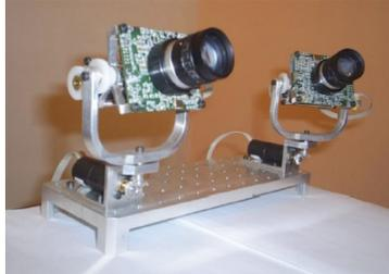
Figure 1: The active visual system constructed for this research work.
