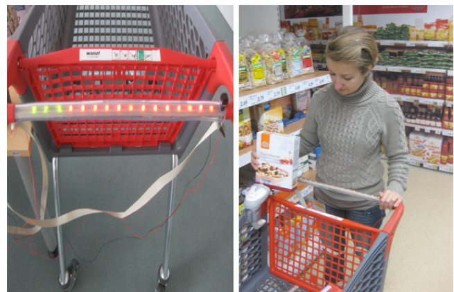
Figure 1. The Augmented Shopping Trolley display consists of 16 LEDs embedded in the handlebar, each of which can be set to green, red or orange
